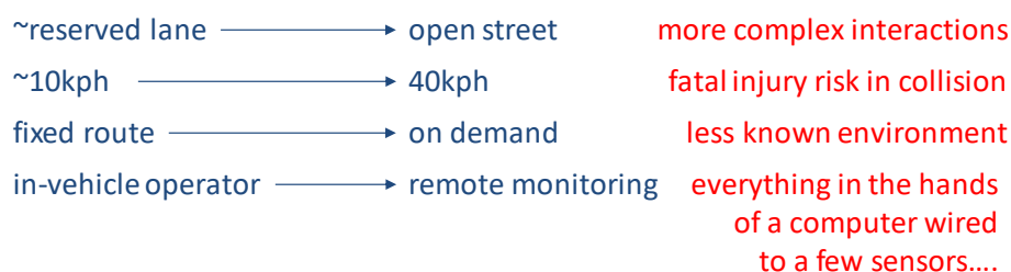
Figure 1. Automated minibuses safety challenges
